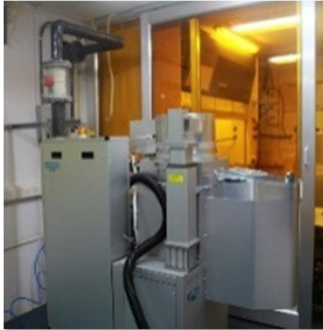
Figure 5.9: ICP-RIE Sentech SI-500 system
