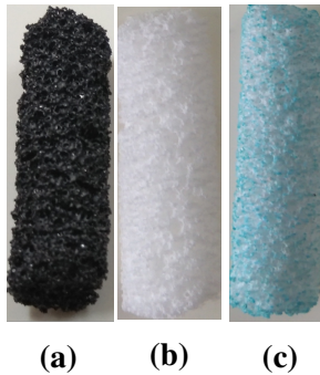
Figure 5.1: a) Foam obtained before sintering. b) Foam after in-situ hydrothermal synthesis. c) Foam obtained after ion exchange with copper acetate.
