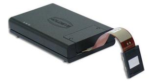
Figure A3.1: Photograph of Pluto phase only SLM
