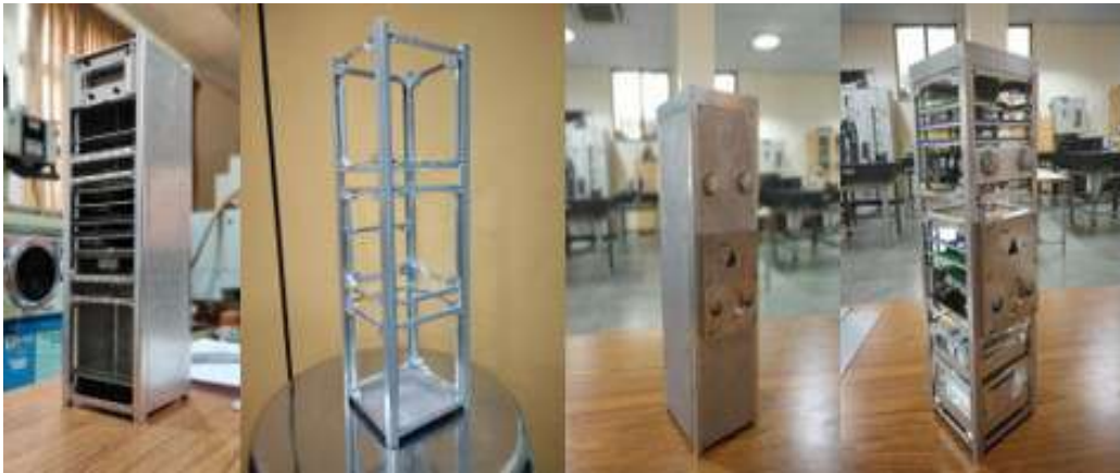
Leftmost Image is the mass dummy developed for Ahan satellite and the rest of 3-images are the structure, and mass dummies developed for AAReST mission
